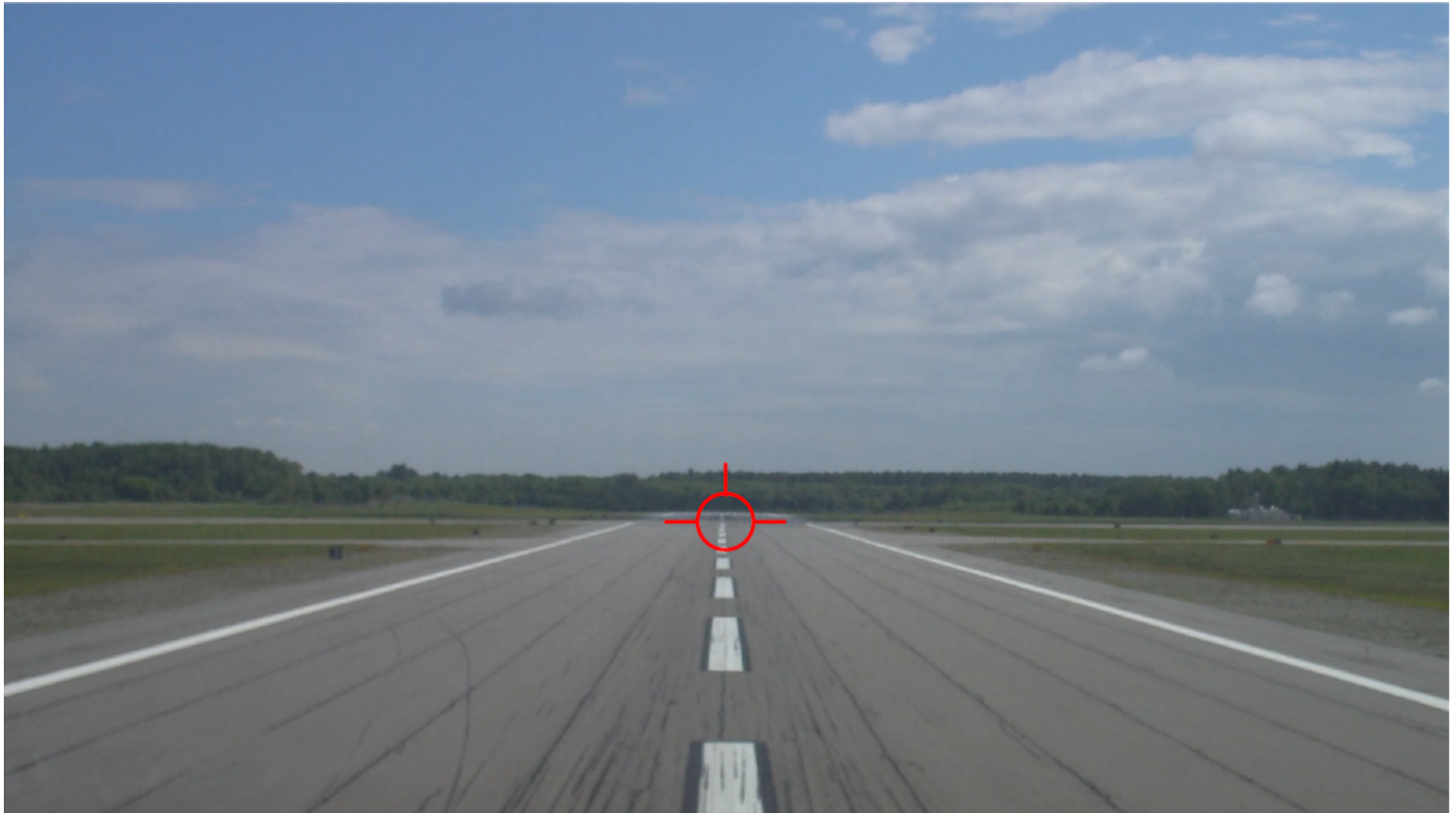
A G450's flight path vector at 10 ft. on a short runway (KBED Runway 23). Photo credit: James Albright
