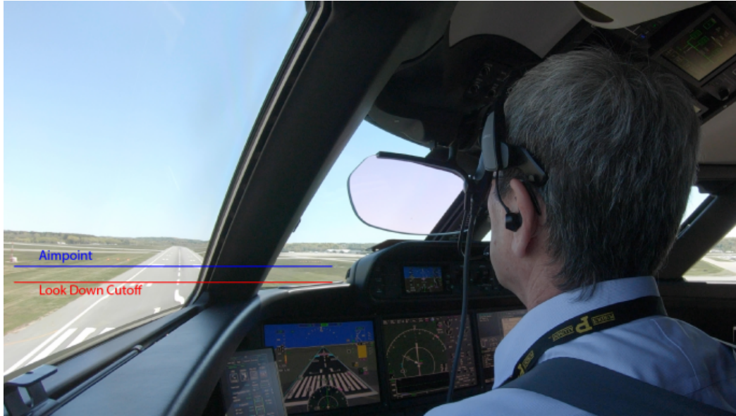
GoPro view of the author's GVII at 25 ft., showing the cutoff point is 500 ft. short of the aimpoint. Photo credit: James Albright
