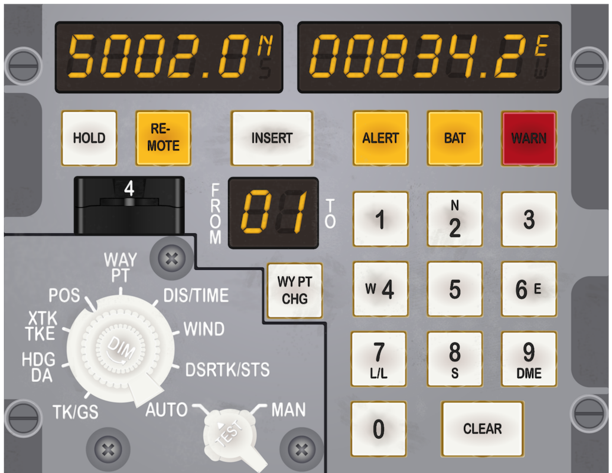
A Delco Carousel IV navigation system. Drawing: Marvin Mutz
