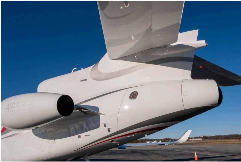
The “S-duct,” which moves air from above the fuselage aft and down to the center engine. Credit: James Albright
