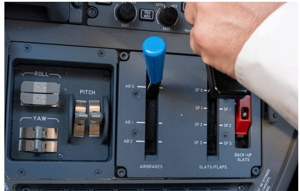
The airbrakes and slats/flaps handles. Credit: James Albright
