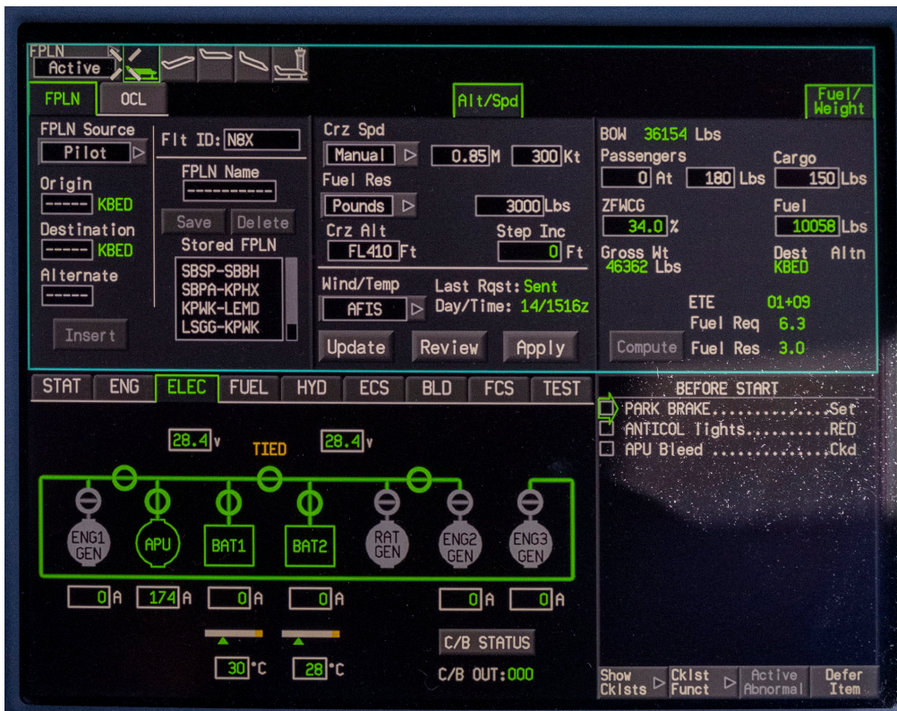
The flight plan and electrical system synoptic prior to engine start.
