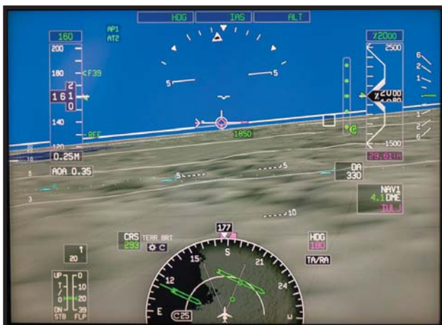
Gulfstream G450 synthetic vision showing right base looking at 4, 5, and 6 mi. to go markers
