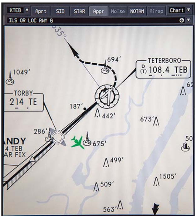
The Teterboro ILS 06 circle to 01 as seen from a Gulfstream G450 cockpit chart display
