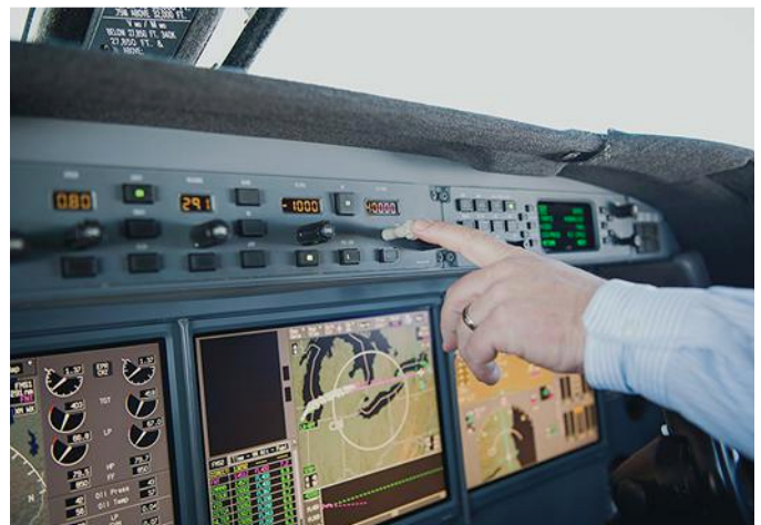
The PM announces the altitude change while pointing to the Altitude Selector
