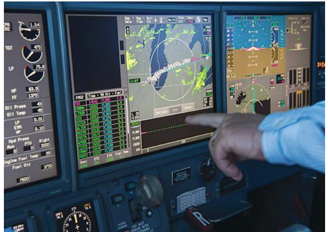
PM points to the "Activate" prompt prior to a navigation course change
