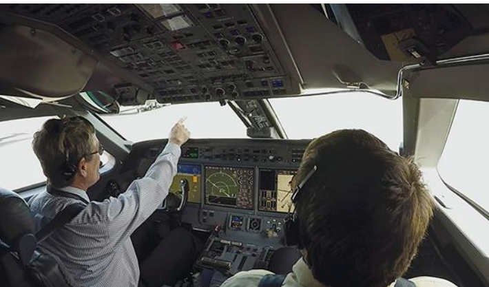
Pilot identifies (the point) and announces (the call) the next taxiway sign
