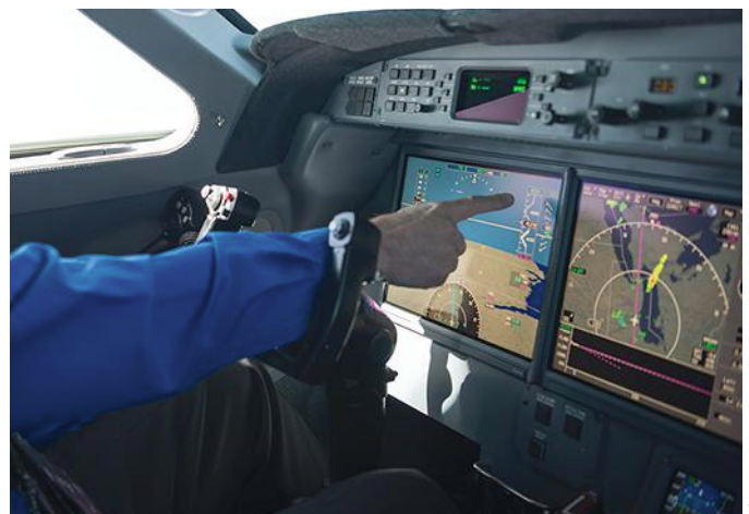
The PF repeats the altitude change while pointing to the selected altitude on the primary display
