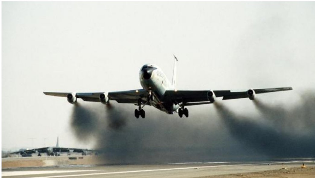
A Boeing KC-135A tanker takeoff with water injection. Credit: U.S. Air Force
