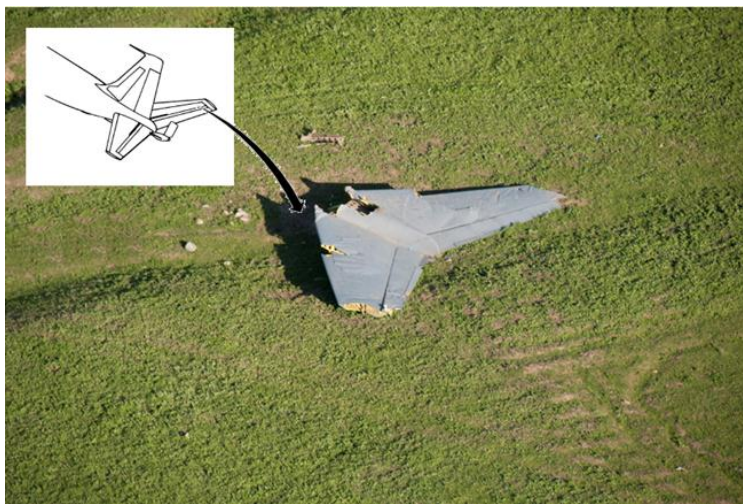
Figure 15. Horizontal Stabilizer Sections and Portion of Aft Fuselage (Tab Z-8)
